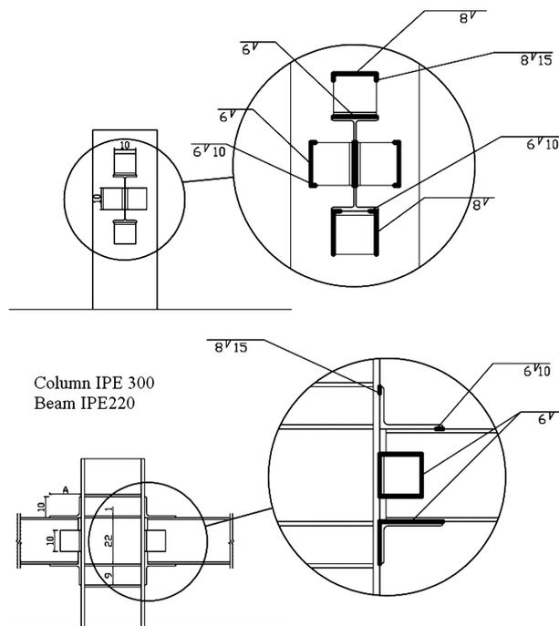
Figure 3. Specimen details for the SWW connection group.
