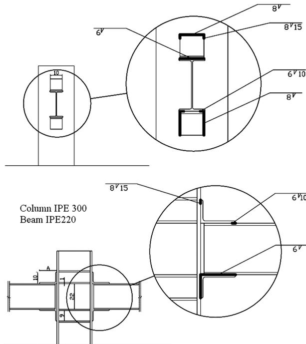
Figure 2. Specimen details for the SOW connection group.
