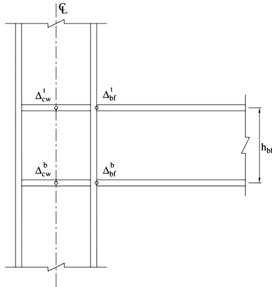
Figure 1. Definition of joint deformation components.
