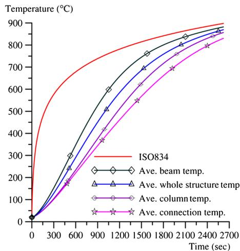
Figure 9. Temperature profiles of each region of connection (Mao *et al.*, 2009).
