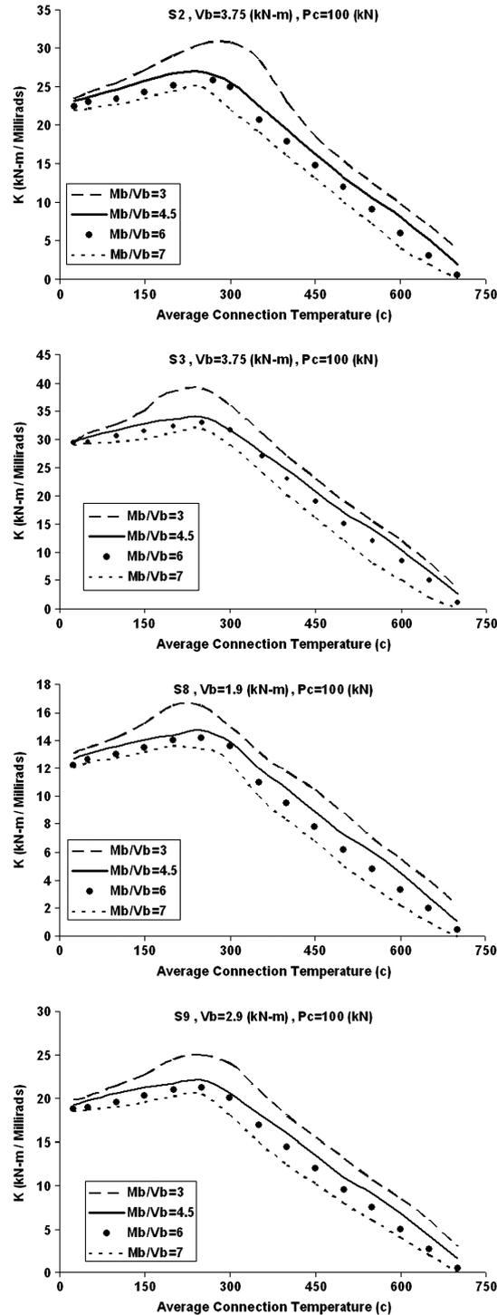
Figure 18. Effect of applied moments on connection stiffness.
