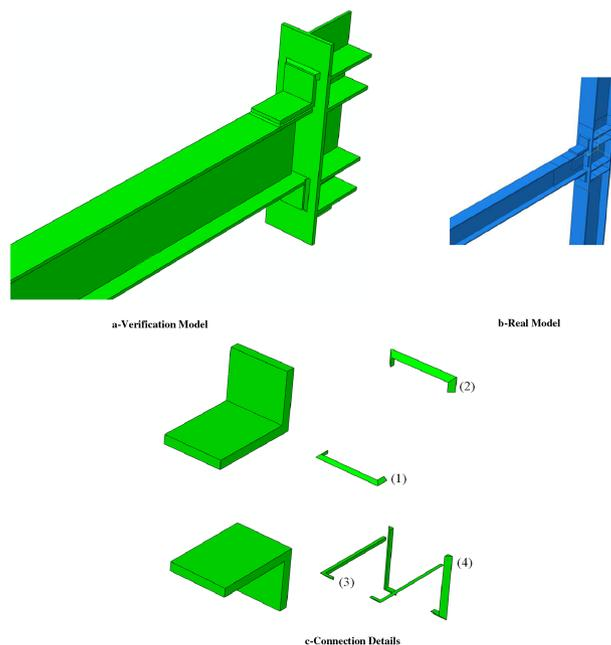
Figure 4. Finite element model of the connection. (a) Verification model. (B) Real model. (C) Connection details.
