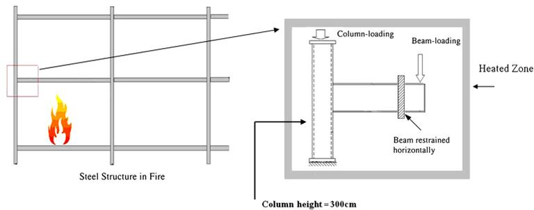
Figure 8. Boundary conditions and applied loads in the second part.
