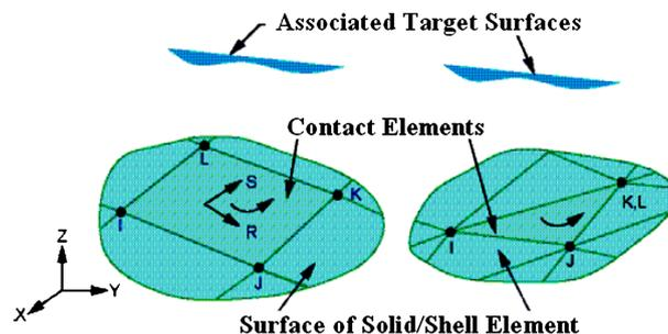
Figure 5. Surface-to-surface contact element.
