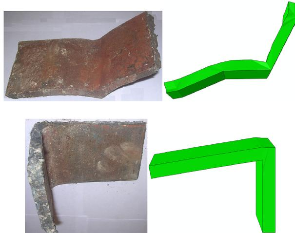
Figure 13. Detail of deformation of the connection S2 components.
