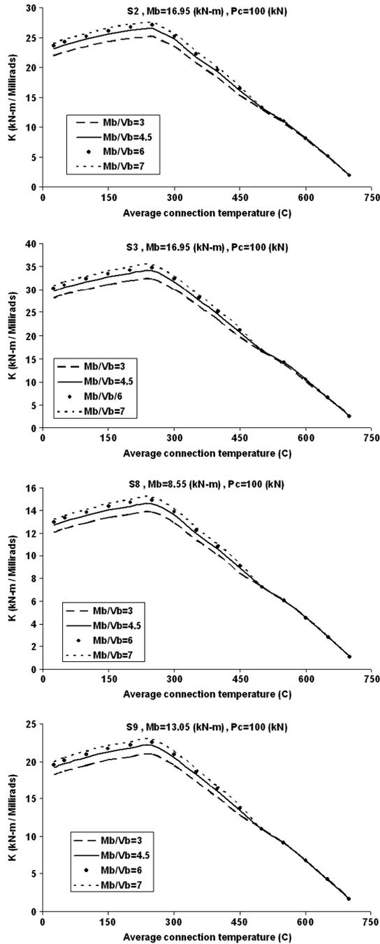
Figure 19. Effect of shear forces of beam on connection stiffness.
