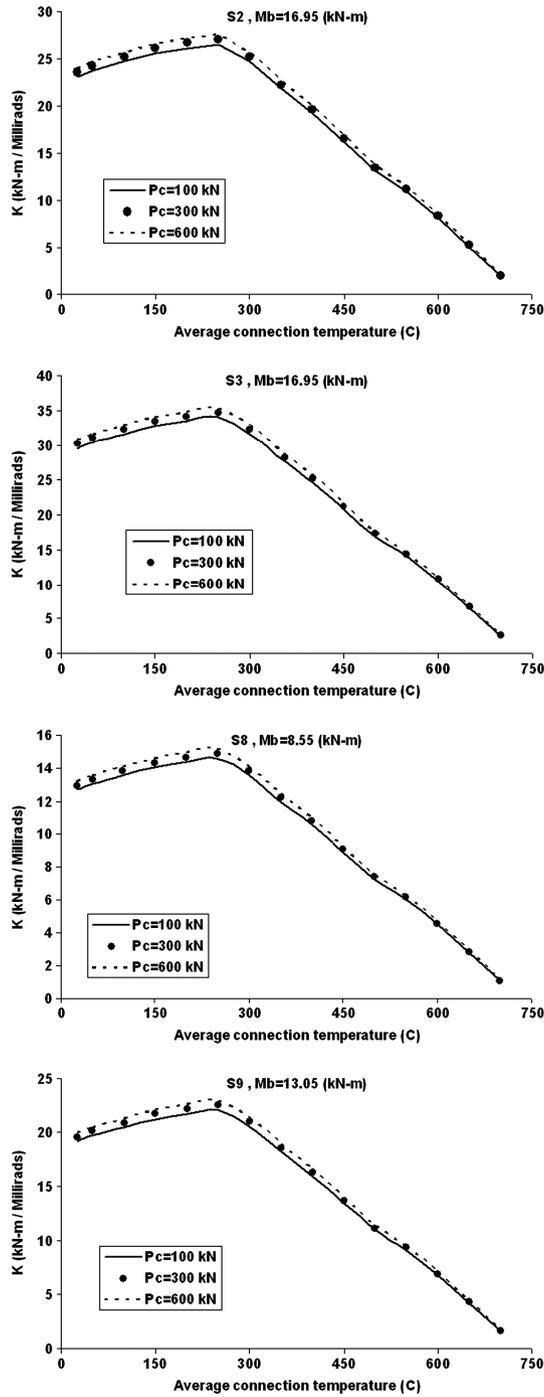
Figure 17. Effect of axial load of column on connection stiffness.
