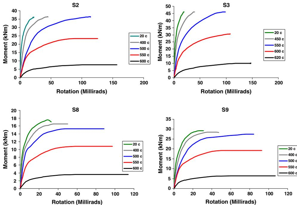
Figure 15. Moment–rotation–temperature curves.
