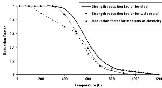
Figure 10. Reduction factor at elevated temperature.
