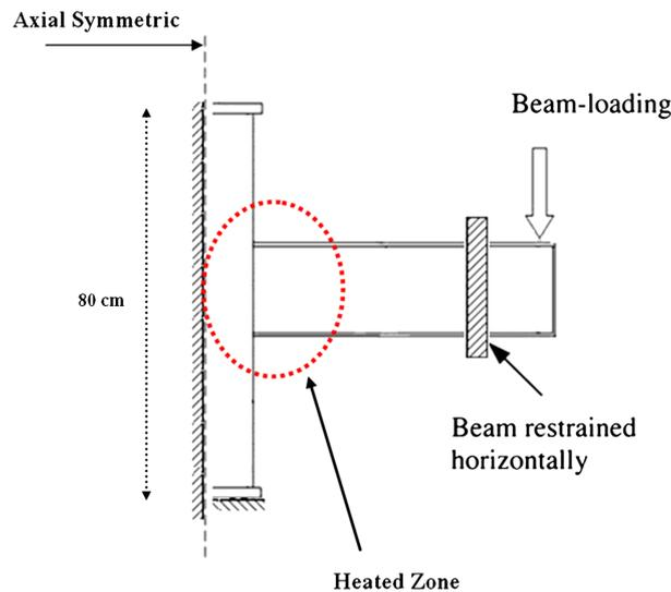
Figure 6. Boundary conditions and applied loads in the first part.
