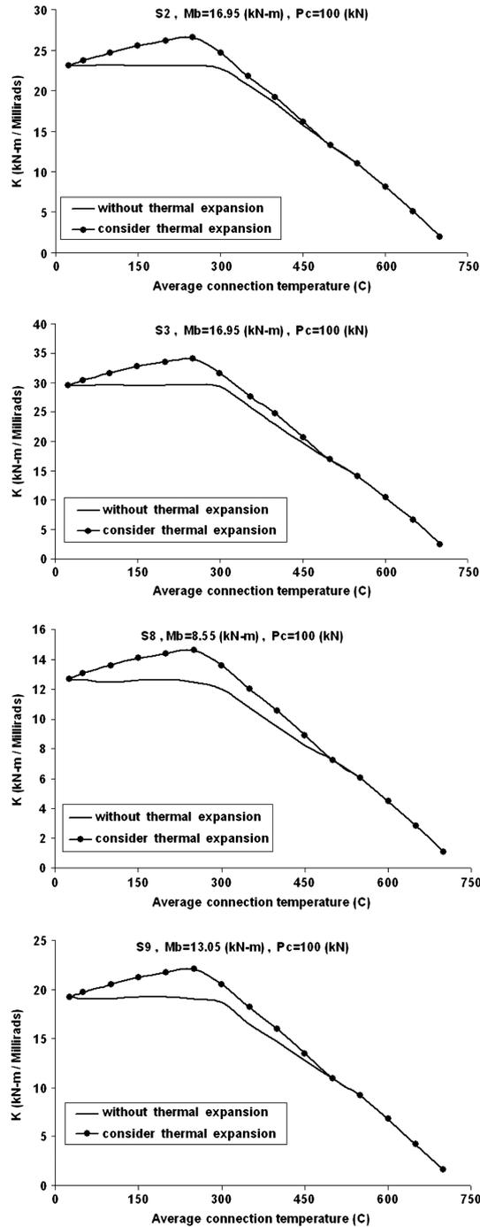
Figure 16. Effect of thermal expansion on connection stiffness.
