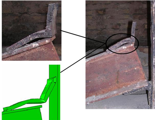
Figure 11. Deformation of the beam-to-column configuration. Connection S2.
