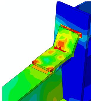
Figure 12. Predicted deformation of the beam-to-column configuration. Connection S2.
