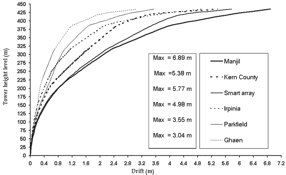
Figure 8. Tower displacement in the X direction
