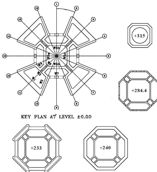
Figure 2. The cross-section of the concrete shaft at different elevations
