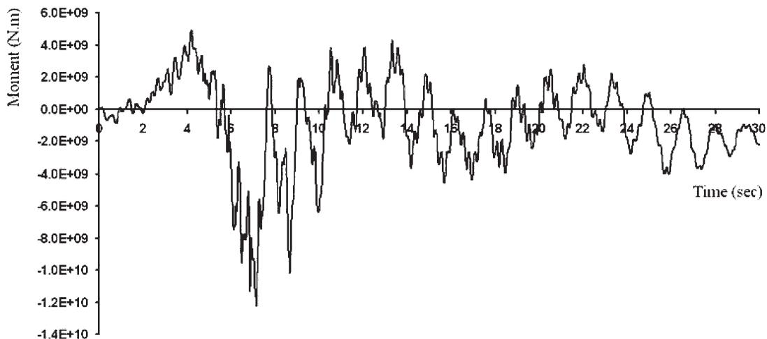
Figure 7. Base moment-time history in the *Y* direction due to the Smart Array earthquake
