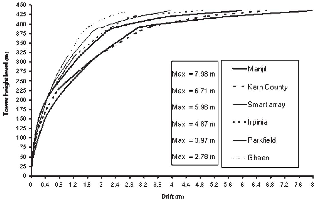
Figure 9. Tower displacement in the Y direction
