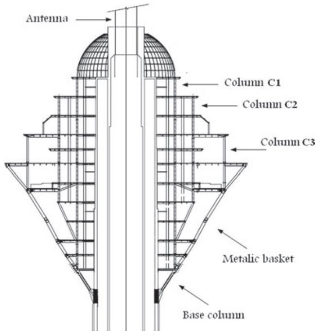
Figure 3. The head structure of Milad Tower
