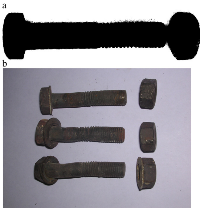
Fig. 15. Second mode of tension failure: (a) specimen in Kerby tests, (b) the specimen in the current study.
