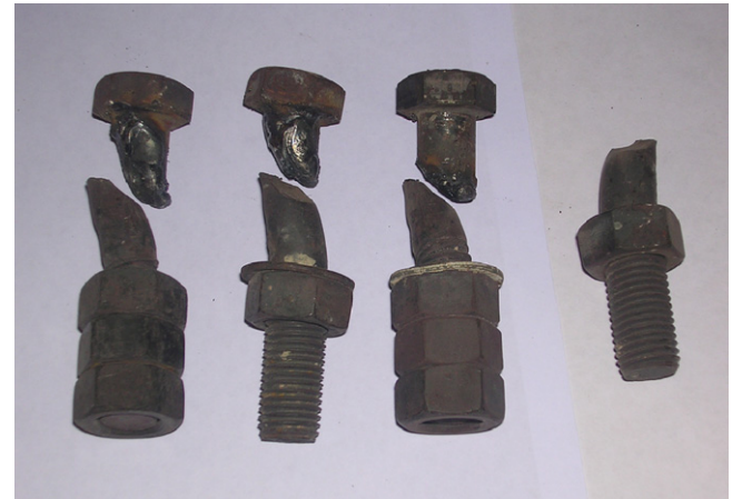
Fig. 16. Shear failure of bolts in the current study.
